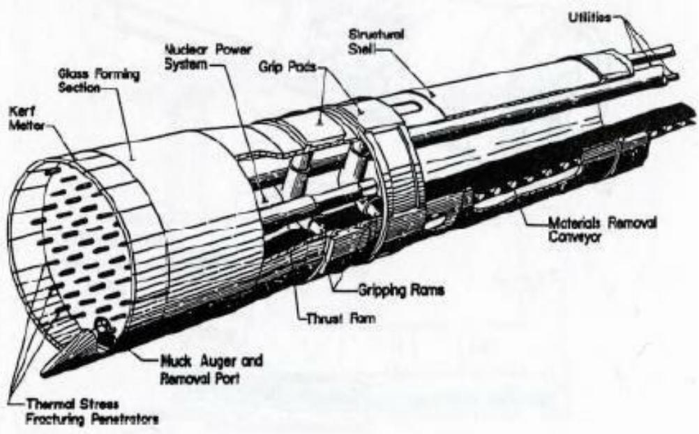
Two Types of Nuclear Subterranean Boring and Excavating Machines<sup>52</sup>
