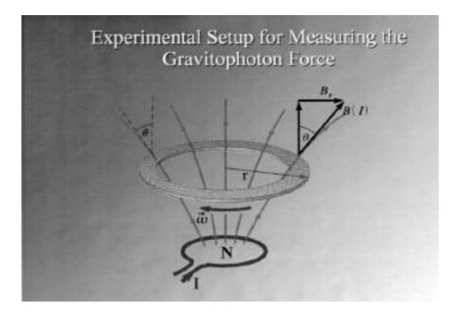
Dröscher and Häuser's Proposed Apparatus for the Testing of a Field Propulsion Principle in a Plane Parallel to the Axis of Two Stacked Counter-rotating Systems
