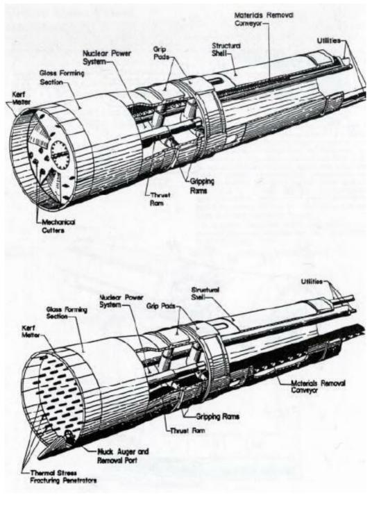
Two Types of Nuclear Subterrene Boring and Excavating Machines<sup>52</sup>
