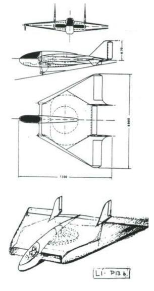
The large air intakes for the ramjets and the disk-shaped combustion chamber are clearly evident. Wind tunnel trials soon showed the advantages of the pure delta shape for supersonic flight, however, and Lippisch produced his final design for the P13b, the final design for which is described in a U.S. intelligence summary for April, 1945:
